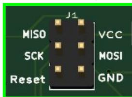
The ISP header consists of 2x3 pins.
